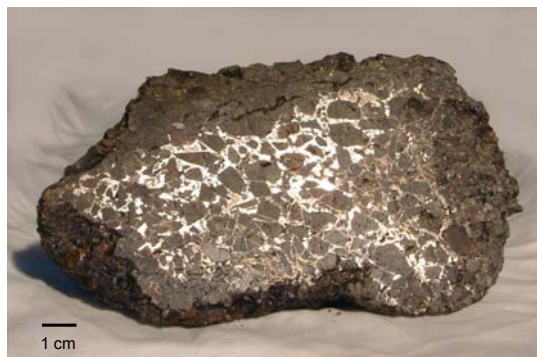
Figure 1. Optical image of the 1.5kg sample as deposited at the OU, note the contrast between the bright metal areas and the dull orange coloured sulphide regions.
