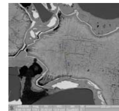
Figure 5 SEM BSD image of oxidised plessitic kamacite rimmed with taenite
